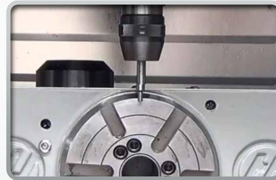
Edge find the platter with the A axis @ 90^\circ
